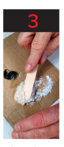
Ensure both parts are being dispensed. Keep the 2-parts of the adhesive separate. Dispense the same amount of additive as the activator (black) and mix in with the white part using a tongue depressor. When thoroughly mixed add in the activator (black part). Continue mixing until all components are thoroughly mixed together.
